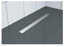
8. Once the liquid foil is completely dry as per the manufacturer's instructions the shower surface can be tiled (eg. ceramic tiles or granite). Seal the gap between the tiles and the channel frame with flexible sanitary sillicone.
